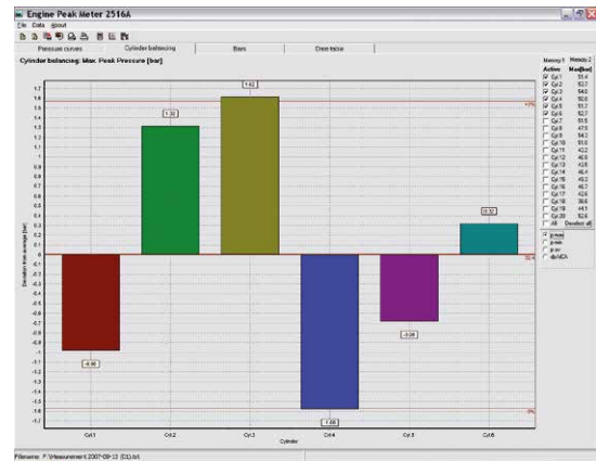
Fig. 3: Cylinder peak pressure deviation p_{av} of each individual cylinder compared to the calculated average peak pressure of the engine, before and after the maintenance work ("as found" / "as left")
